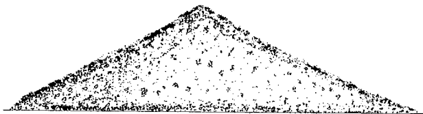
c) Aggregate saturated surface-dry; almost complete collapse but definite peak still visible and slopes are angular
