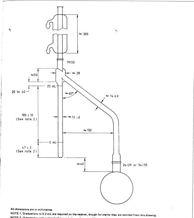
NOTE 2. If apparatus with a glass bulb is used, then a dimension 30 mm to 60 mm may be used in place of 47 ± 2 mm and 170 mm to 210 mm in place of 180 ± 10 mm, provided the graduations in the upper tube allow for the precision tolerances in F.7 to be achieved.
